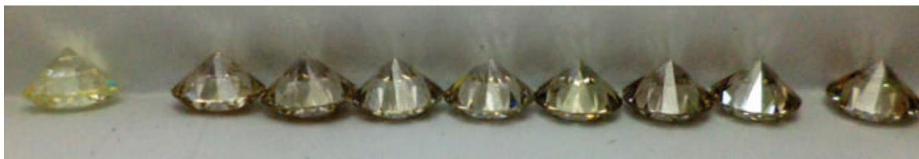
Fig 2: Distinct brownish tint was observed for all the synthetic CVD diamonds
