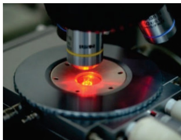
Fig.2.PL measurement of a diamond with 633nm red laser excitation
