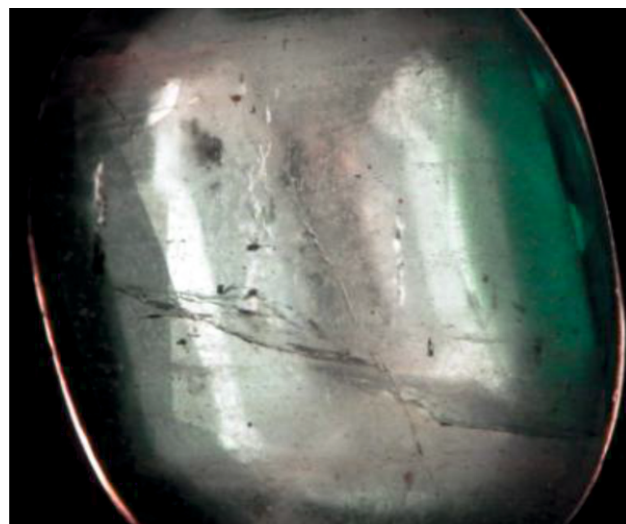
Fig.6: Fluid and crystalline inclusions in table portion
