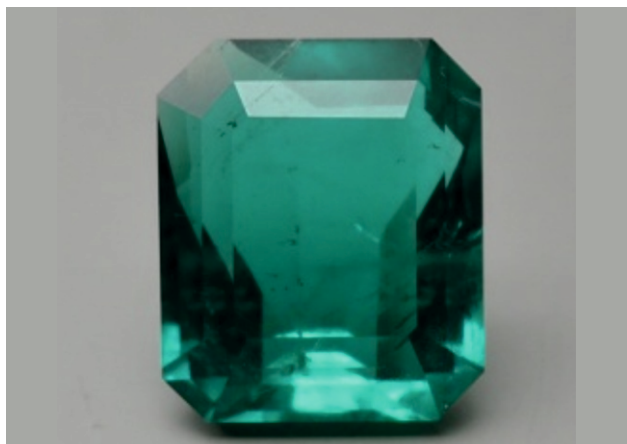
Fig 1 and Fig 2: The 4.75ct hydrothermal synthetic emerald submitted for identification to Hanmi lab
