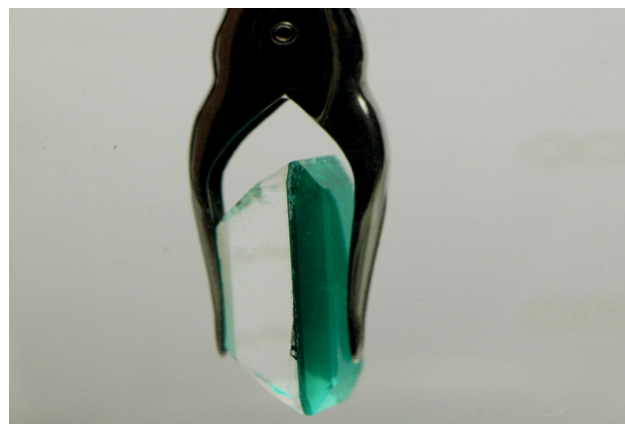
Fig.3. Colourless pavilion layer as seen here when the doublet was immersed in water (Photo by Tay)
