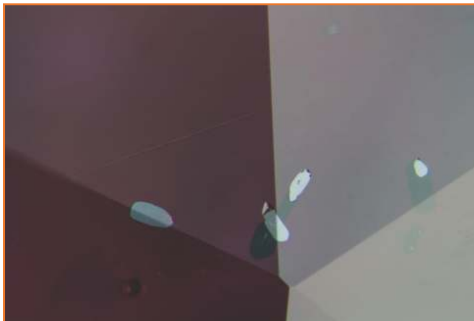
Fig 6 When observed in reflected light the metallic lustre of the primary rutile present on the surface.
