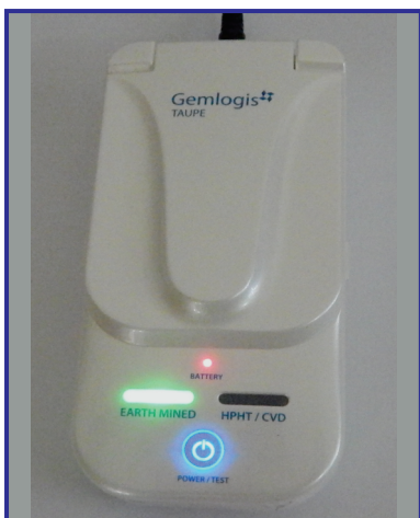
Fig 5 : Green glow seen for irradiated Synthetic CVD
