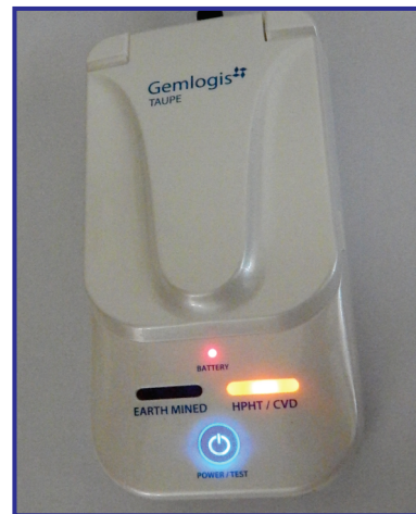
Fig 6 : Yellow orange glow for irradiated Synthetic HPHT diamond
